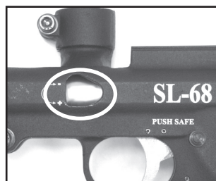
Figure 5: Cleaning Port Location
